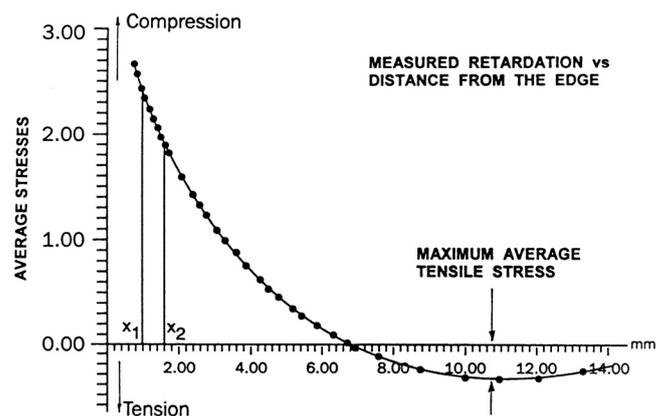
and laminated glass [1]. As shown in figure 2, the edge surface of a glass "E" will develop surface compression comparable in size [2] to the surface (F) stress, assuming the cooling rate and the heat flow are approximately the same.
